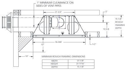
A wall, Perpendicular and in front of this appliance's glass door face must be at least 12" away from the side edges of the glass frame. A wall at 45° angle to the front face and starting at the side edge of this appliance is allowed. Projections behind this 45° angle edge (shaded area) are allowed.
